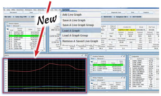
Setting up the 'LIVE GRAPH' is easy. The technician can setup different 'LIVE GRAPHS' to monitor different sensors, save each 'LIVE GRAPH SETUP' and than save them in a 'GROUP' file and load them into your work space each time you view the controller you are connected to.
