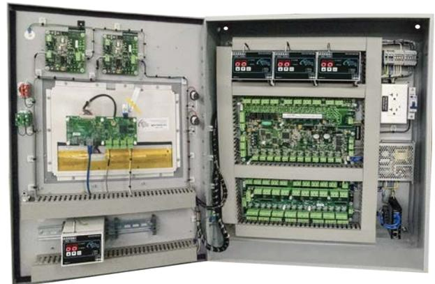
Input power supplied to the enclosure can be 115/230 volts, and using a MCS Power Supply is converted to 12 volts to power all the boards in the enclosed above.
