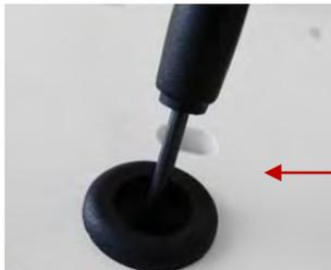
Puncture a small hole in the grommet on the back side of the thermostat. You want the wires to be tight so no air passes through affecting the thermostat's reading.
