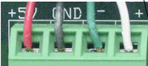
Enlarged view of Thermostat block wiring
