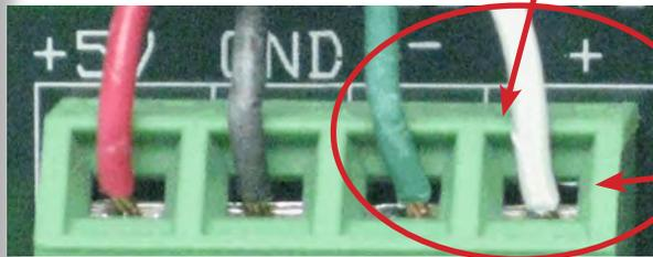
Enlarged view of Thermostat block wiring
