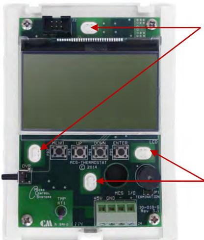
Using a 1/4" Phillips screwdriver, insert one of 1/4" machine screws into one of the mounting slots depending on the J-box you are utilizing and tighten the screw to hold the mounting wall plate into position.
