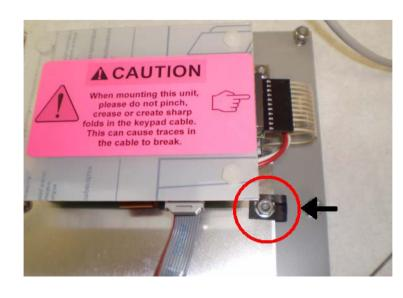
When mounting the MAG-KEYPAD, fold over the black ground tab on the right side of the Keypad, and place the washer over the black tab. Fasten the nut on the Keypad.
