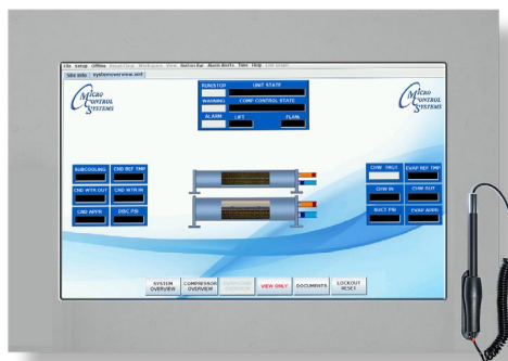
EVAPORATOR CONDENSER OVERVIEW SCREEN
