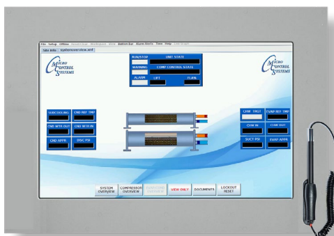
EVAPORATOR CONDENSER OVERVIEW SCREEN
