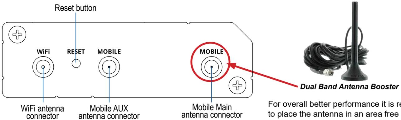
For overall better performance it is recommended to place the antenna in an area free of obstructions and interference, such as outside or at an elevated position.
