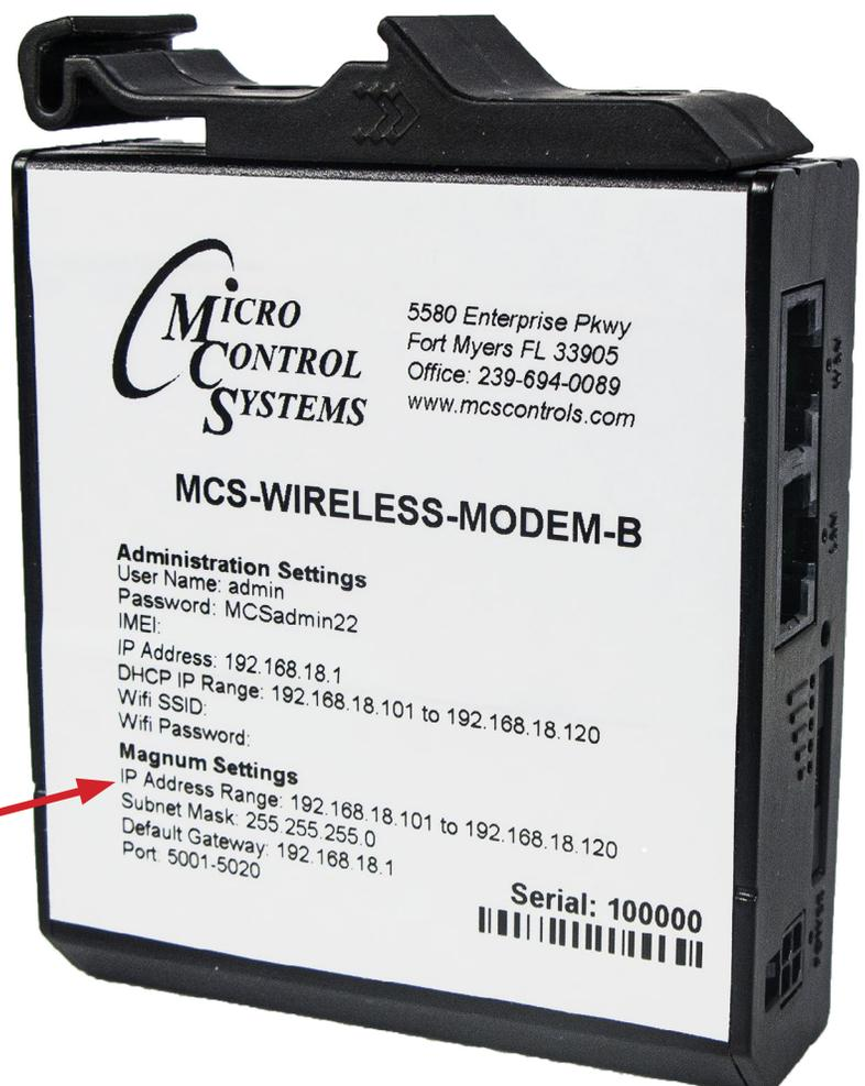
MAGNUM IP must be within the specified IP address range on the label.
