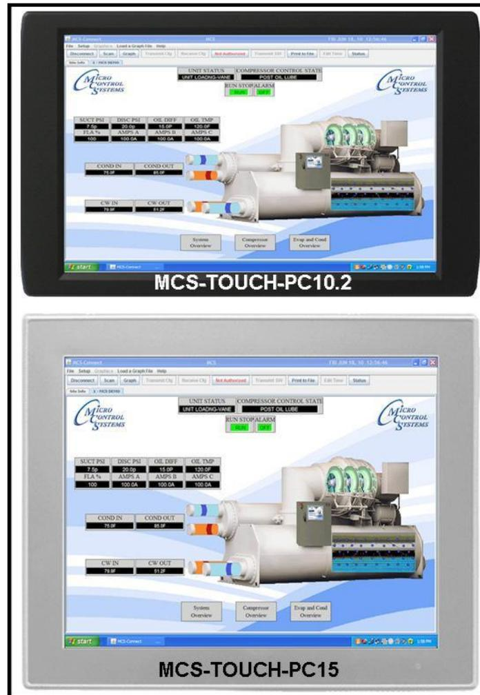
The MCS-Touch is capable of saving Offline History Files containing detailed operational data when connected to the MCS-Magnum or MicroMag. Extended History Saving can be set to active when the MCS-Touch is in idle mode and will create a new history file for every 16 minutes of operation.
