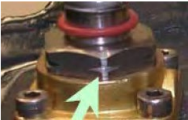
NORMALLY OPEN SOLENOID CAN BE IDENTIFIED BY NOTCHES ON NUT
