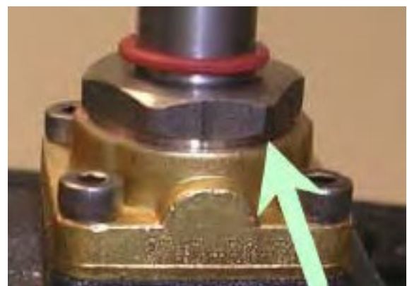
NORMALLY CLOSED SOLENOID THERE ARE NO NOTCHES ON THE NUT
