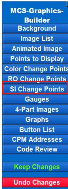
1. 'SI CHANGE POINTS TAB' - Used for Digital sensors, displays an image for each state (Auto, On, Off). If set to editable, it can be used to change the state of the sensor if auth level is reached.
