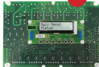
LCD mounted on back of MicroMag with new Standoffs
