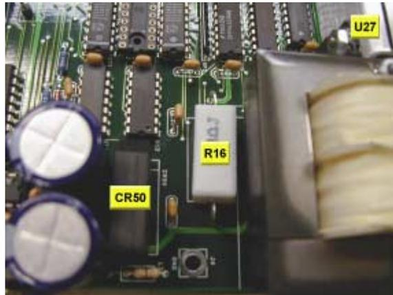
To determine if the loss of Vaa is due to a broken foil trace, simply remove power to the board and measure for continuity between pin 3 of U27 (pin 3 is the pin closest to the power transformer) and the end of R16 closest to the edge of the board. If you do not measure continuity, the trace is broken. If you do measure continuity, the trace is intact and your board will require factory service.
